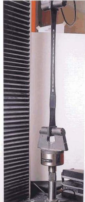
Each delivery is tested for tensile strength, elongation and other properties, including seam strength.
