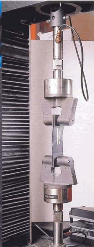
Each delivery is tested for tensile strength, elongation and other properties, including seam strength.
